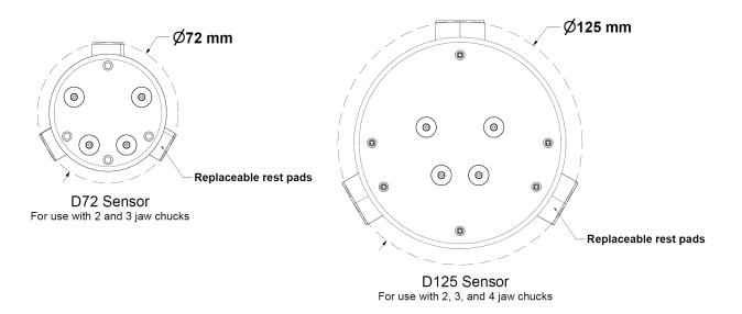
The Kitagawa Europe wireless chuck force gauge is designed to quickly and accurately measure holding force and speed on chucks. Verifying chuck holding force allows manufacturers to improve the repeatability of a manufacturing process by checking actual holding force under dynamic (rotating) conditions, as well as perform critical preventative maintenance checks.
